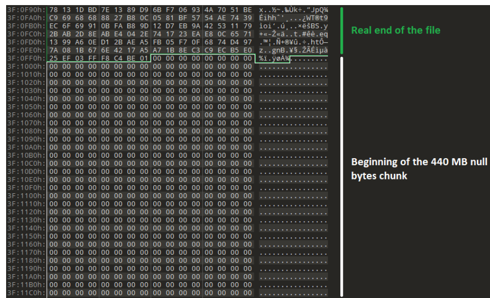
Figure 9 Beginning of the 440 MB null bytes chunk in the setup.exe sample.
